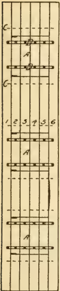
FIG. 173. Six-stave silo front, ready to be put up; A, A, A, A, doors; C, C, C, dowel pins; D, D, D, door battens (Cap. Lbr. Co.)
